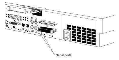
Figure 5-11 Serial Ports on the Rear of the Indy Workstation
