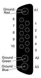
**Figure A-13** Graphics Port Pinout Assignments
