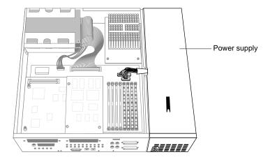
Figure 8-37 Locating the Power Supply
