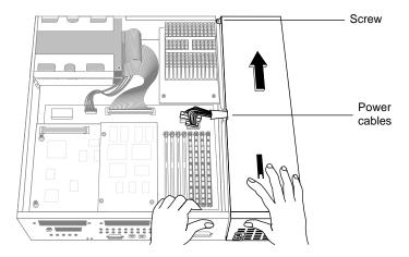
Figure 8-38 Removing the Power Supply
