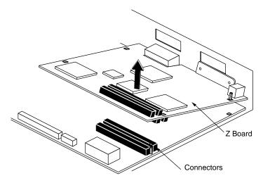
Figure 8-19 Disconnecting the Z Board From the System Board
