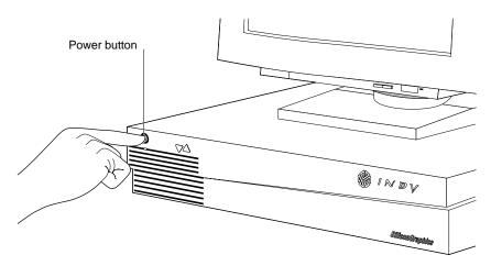
Figure 2-7 Turning on the Indy Workstation
