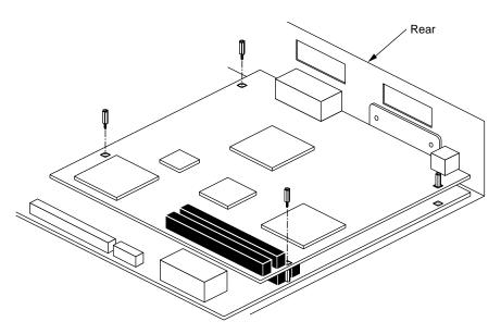
Figure 8-17 Removing the Standoff Screws From the Z Board
