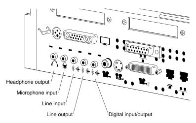
Figure 5-13 Connecting an Audio Device to the Indy Workstation
