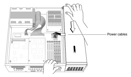
Figure 8-39 Installing the Power Supply
