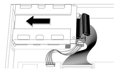
**Figure 5-4** Installing the Floptical Drive Above the System Drive
