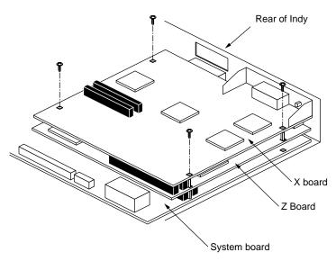
Figure 8-14 Removing the Screws From the X Board
