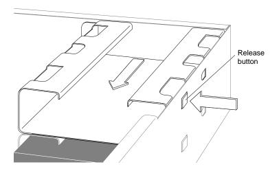
Figure 5-2 Removing the Drive Bracket
