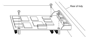
Figure 4-5 Installing a Single-Width GIO Option Board
