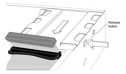
Figure 8-31 Removing the Floptical Drive and Bracket
