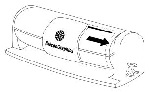
Figure 2-20 Sliding the IndyCam Lens Cover Aside
