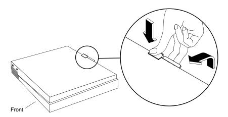
Figure 2-28 Removing the Top Cover From the Indy Workstation
