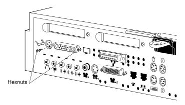
Figure 8-13 Replacing the Screws on the Graphics Board's I/O Connector
