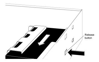
Figure 8-33 Removing the System Disk Drive
