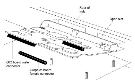
Figure 4-4 Positioning a Double-Width Board
