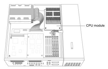
Figure 8-20 Locating the CPU Module
