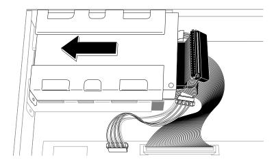
Figure 8-36 Re-installing the Floptical Drive
