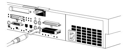
**Figure 5-12** Connecting the Serial Cable to the Serial Port
