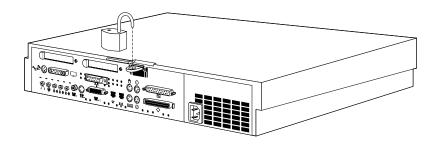
Figure 2-30 Attaching a Lock to the Indy Workstation
