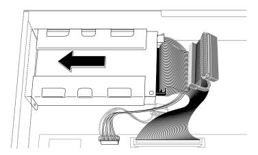
Figure 8-35 Installing the Replacement System Disk Drive
