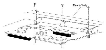
Figure 4-6 Installing a Double-Width GIO Option Board
