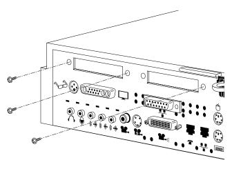
Figure 8-4 Removing the External Screws From a Double-Width Board
