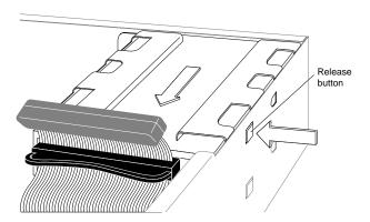
Figure 8-28 Removing the Floptical Drive
