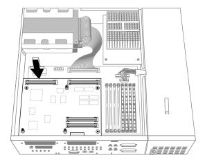
Figure 8-11 Connecting the Graphics Board to the System Board
