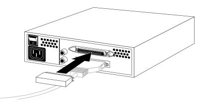
Figure 5-8 Connecting a Terminator to the Last SCSI Device on the Daisy-Chain
