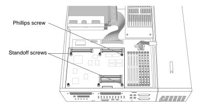
**Figure 8-9** Removing the Screws From the Graphics Board
