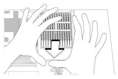
Figure 8-23 Installing the CPU Module
