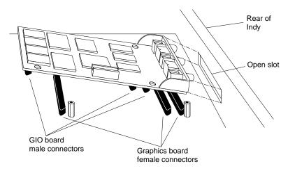
Figure 4-3 Positioning a Single-Width Board
