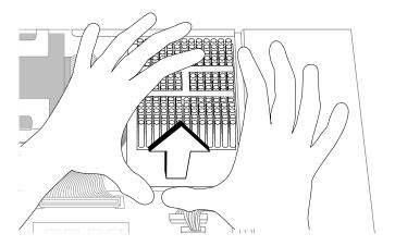
Figure 8-22 Disconnecting the CPU Module
