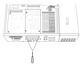
**Figure 8-3** Removing the External Screws From a Single-Width Board
