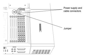
Figure 7-12 Locating the Password Jumper
