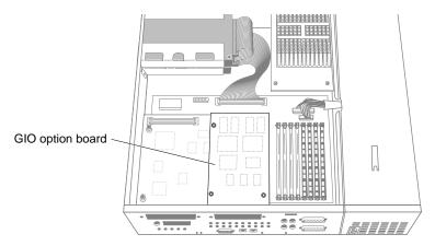
Figure 3-5 The GIO Board Installed on the Right Side of the Graphics Board
