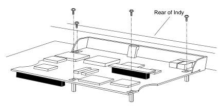
Figure 8-6 Removing the Screws From a Double-Width GIO Option Board
