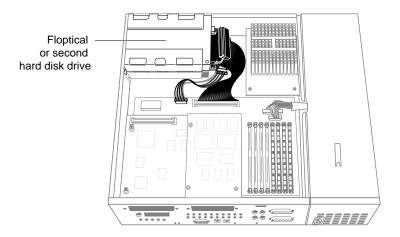
**Figure 8-30** Locating the Floptical Drive Installed in the Top Slot
